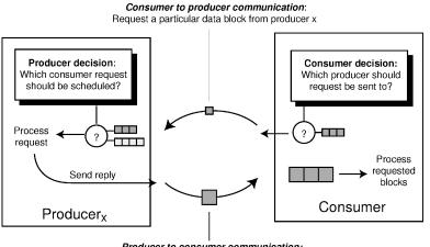
Producer to consumer communication: Reply to request with data block
