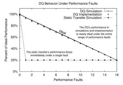
Fig. 9. **Distributed queue performance:** results from a simulation of DQ and an implementation of the DQ are presented, and compared to ideal performance under an increasing number of performance faults, as well as to the performance of a "static transfer." In the experiments, producers generate data at 40 MB/s and nonfaulty consumers consume data at 5 MB/s. A performance fault reduces a consumer's performance by a factor of 5, down to 1 MB/s.
