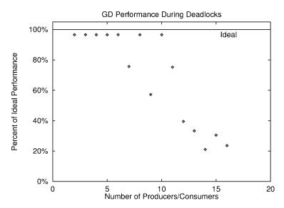
Fig. 18. **Switch deadlock:** performance of graduated declustering plotted under scale, in cases where the switch deadlock would occur. In the graph, the number of producers and consumers is covaried along the *x*-axis, and the percent of ideal performance is plotted along the *y*-axis. Thus, at x = 16, there are 32 machines involved in the experiment. The deadlock only occurs at scale and higher rates, but when it does occur, performance drops noticeably.
