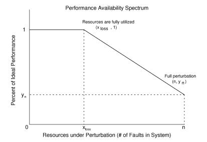
Fig. 8. **Performance availability spectrum:** overall performance under an increasing number of performance faults. Along the *x*-axis, the number of components experiencing the performance fault is increased up to the maximum number of components in the system n. Overall system performance, as a fraction of ideal performance in a setting free of performance faults, is plotted on the *y*-axis.
