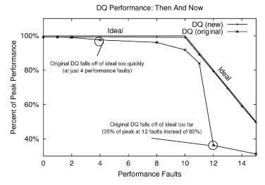
Fig. 1. **DQ performance, then and now:** a comparison of the old DQ implementation versus the new. The number of performance faults is increased along the x-axis, and the percentage of peak performance is plotted along the y-axis. Results from the older version of the DQ are compared against the new and improved algorithm.
