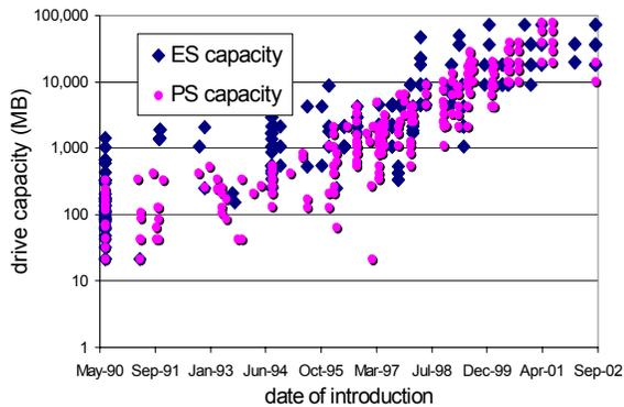
Figure 4: Comparison of capacities. Capacity and introduction date of 10 years of Seagate drives [Seagate02].
