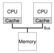
Figure 10.2: Two CPUs With Caches Sharing Memory
