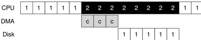
From the timeline, you can see that the copying of data is now handled by the DMA controller. Because the CPU is free during that time, the OS can do something else, here choosing to run Process 2. Process 2 thus gets to use more CPU before Process 1 runs again.
