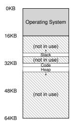
Figure 16.2: Placing Segments In Physical Memory
