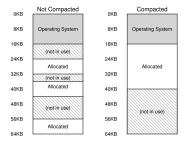
Figure 16.6: Non-compacted and Compacted Memory
