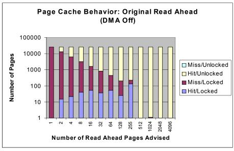
Figure 1: The page-cache behavior with the original read ahead mechanism. As the number of read ahead pages is increased, the number of misses on locked pages decreases as one would expect.
