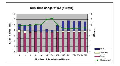
Figure 5: Runtime usage with the read ahead modifications. Idle time is approaching zero for read aheads of 32 and 64 pages (advice levels 6 and 7 respectively).
