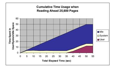
Figure 3: When the current kernel is advised to read ahead 25,600 pages at a time, one observes three periods of activity. From zero to five seconds, almost all of the time is spent in system space. From five to thirty five seconds, almost all of the time is spent in idle space. And from thirty five seconds on, all of the time is spent in user space.
