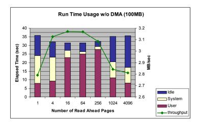
Figure 2: Runtime usage running *mmapit* on a 100MB file with our original Linux configuration. The time spent in user, system, and idle space are displayed for various amount of read ahead pages. The throughput peaks out at only 3.2MB/sec while NTFS peaks at around 13MB/sec.
