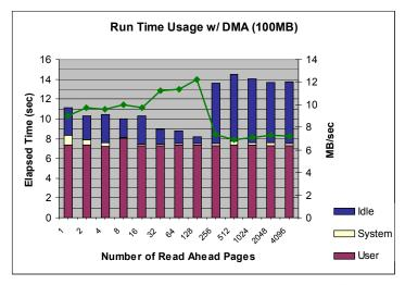
Figure 4: Run time usage for various advise levels and drive DMA enabled. The user time is consistent for each level as it should be. The idle time shows an area to focus on to decrease total elapsed time and increase overall throughput.
