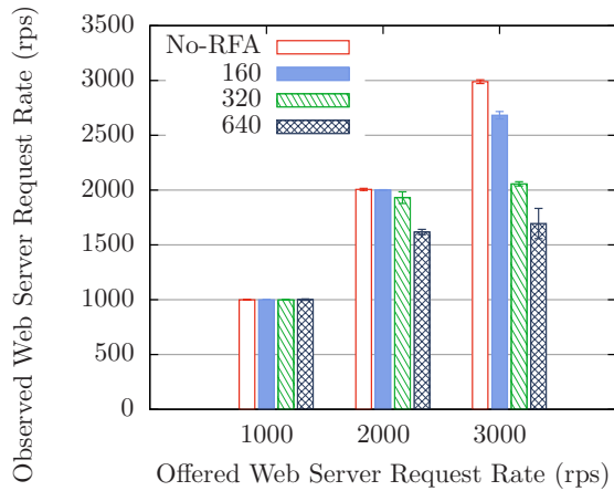
Figure 7: Offered vs. observed load on web server with varying RFA intensities when all the VMs float across all cores.
