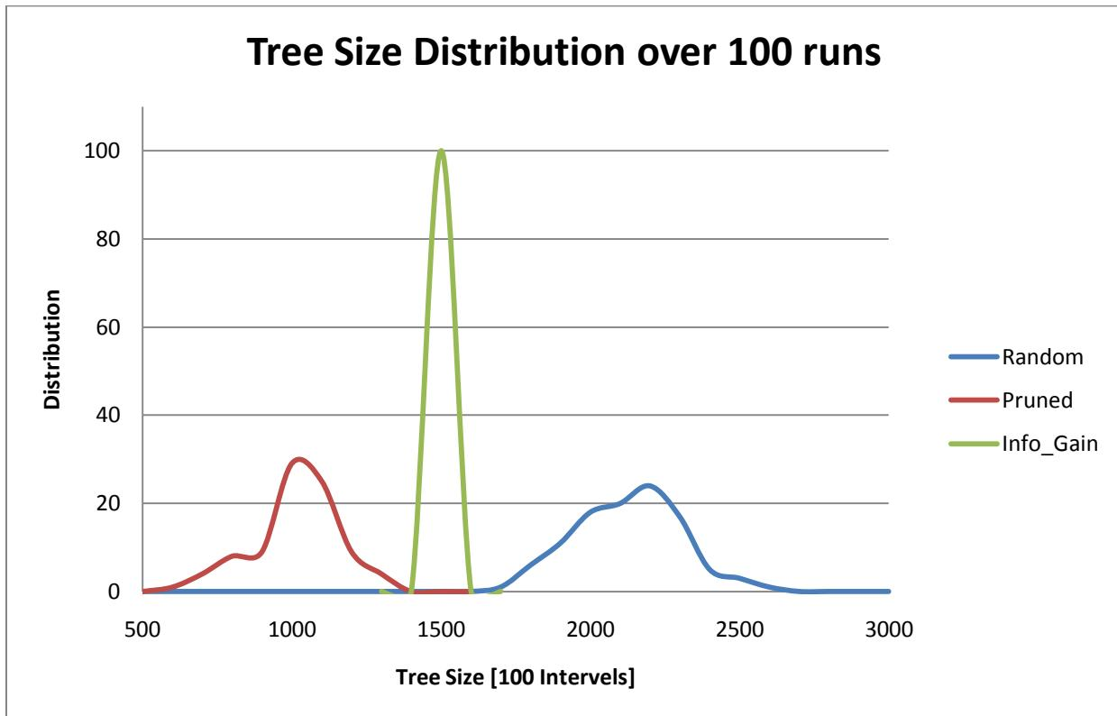
The Pruned method clearly seems generate the smallest trees, size of the Info\_gain trees fall in the middle while the random feature selected tree roughly twice the size of pruned trees. A random feature selected is highly likely to be larger in size than trees generated by prune or info gain.
