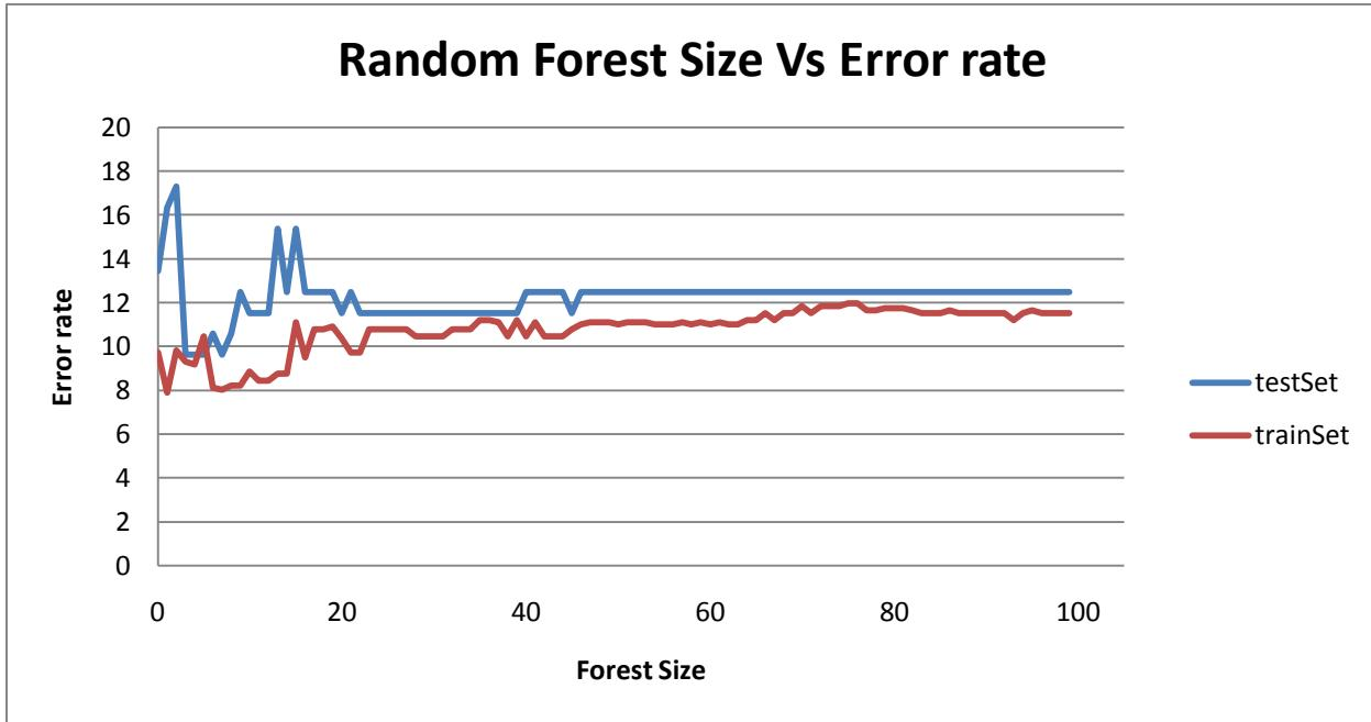
On the Test set error rate seems to converge at forest size 50 for an error rate of 12.5%. The Train set seems to still change a bit but averages around 11.2%
