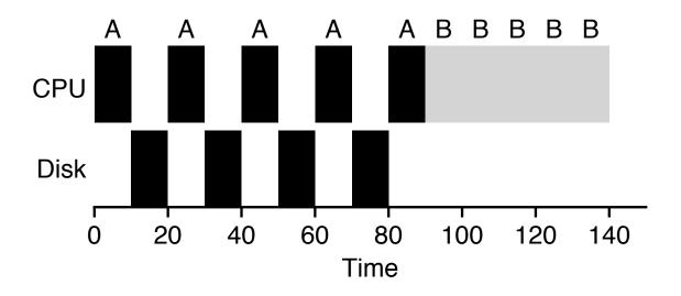
Job holds on to CPU while blocked on disk!
