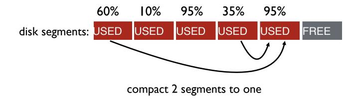
When moving data blocks, copy new inode to point to it When move inode, update imap to point to it
