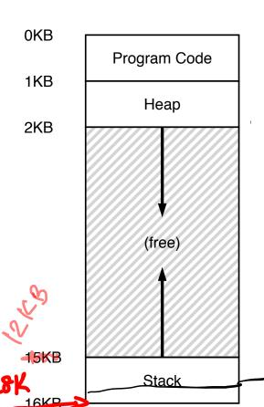
Stack goes  $16K \rightarrow 12K$ , in physical memory is  $28K \rightarrow 24K$ Segment base is at  $28K \rightarrow b$  there is a stack.
