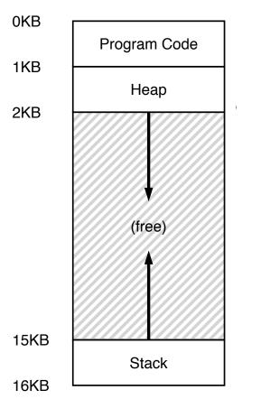
Stack goes 16K  $\rightarrow$  12K, in physical memory is 28K  $\rightarrow$  24K Segment base is at 28K
