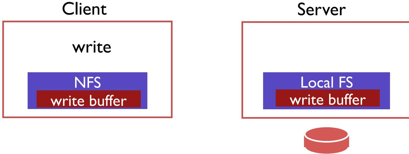
Server acknowledges write before write is pushed to disk;
