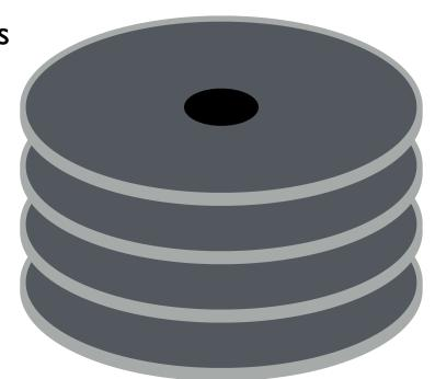
Heads on a moving arm can read from each surface.
