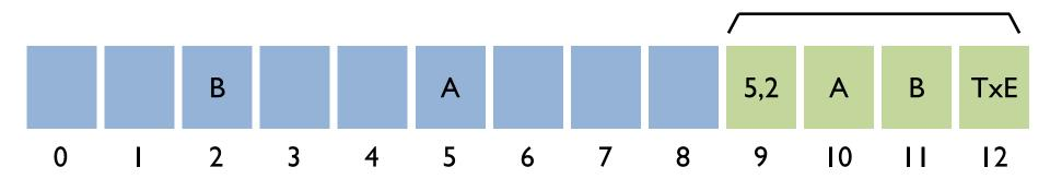
transaction: write A to block 5; write B to block 2 Checkpoint: Writing new data to in-place locations transaction: write C to block 4; write T to block 6
