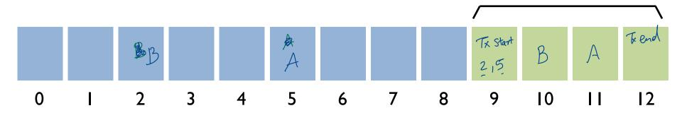
transaction: write A to block 5; write B to block 2 Checkpoint: Writing new data to in-place locations name for this step the step
