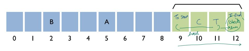
In last transaction block, store checksum of rest of transaction During recovery: If checksum does not match, treat as not valid write order before 9,10,11124,6124,612
