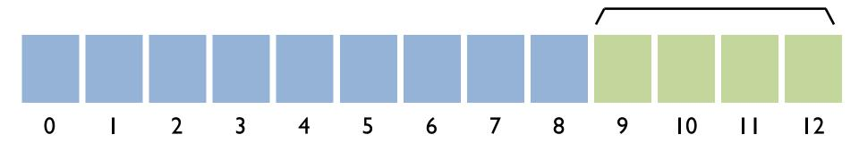
transaction: write A to block 5; write B to block 2 Checkpoint: Writing new data to in-place locations
