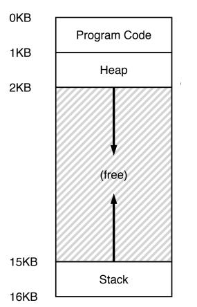
Stack goes  $16K \rightarrow 12K$ , in physical memory is  $28K \rightarrow 24K$ Segment base is at 28K
