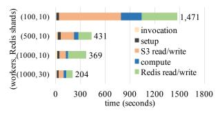
Figure 5: Performance breakdown for sorting 1TB data by how task time is spent on average.
