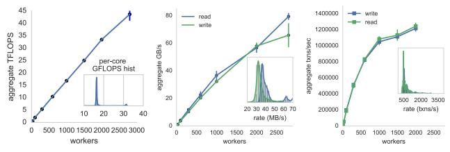
Figure 2: Running a matrix multiplication benchmark inside each worker, we see a linear scalability of FLOPs across 3000 workers
