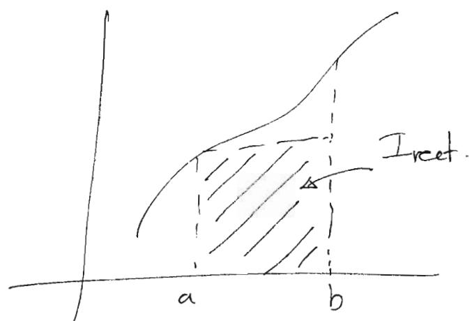
In order to design a "composite" rectangle rule, we use the partition  $a = x_0 < x_1 < \dots < x_{N-1} < x_N = b$ ,
