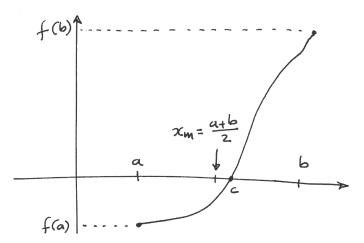
The bisection algorithm attempts to locate the value c where the plot of f crosses over zero, by checking whether it belongs to either of the two sub-intervals  $[a, x_m]$ ,  $[x_m, b]$ , where  $x_m$  is the midpoint
