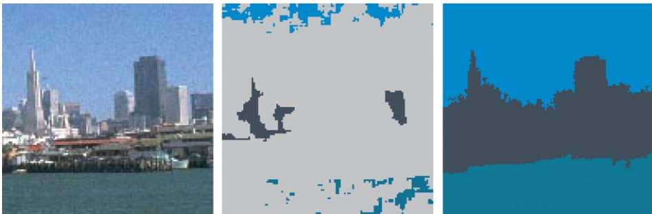
Fig. 12. Segmentation result on the City image: the original image, the initial labelling, and the final segmentation map.
