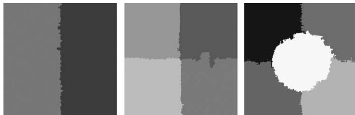
Fig. 17. Segmentation results of the multi-label fast marching algorithm on the synthetic images.
