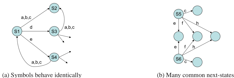
Figure 7.4: Different kinds of transition redundancy in DFAs. ACTs can eliminate redundancy in 7.4a; D 2 FAs are best for eliminating that in 7.4b.
