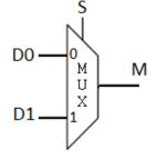
Where **S** is the select line, **D0** and **D1** are the inputs and **M** is the output.
