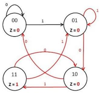
b. Fill out the following **Next State truth table** for the above state diagram where  $S_1$ ' $S_0$ ' represents the next state. (2 **Points**)
