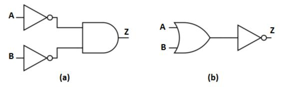
(a) is (NOT A) AND (NOT B) while (b) is NOT(A OR B) These are equivalent by DeMorgan's law.
