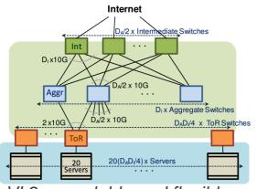
VL2: a scalable and flexible data center network, C. Kim et al., SIGCOMM 2009
