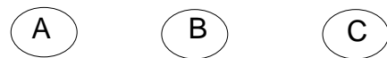
Figure 1: Station B can hear both A and C, but A and C cannot hear each other. A "hidden terminal" scenario results when C attempts to transmit while A is transmitting to B. An "exposed terminal" scenario results if B is transmitting to A when C attempts to transmit.
