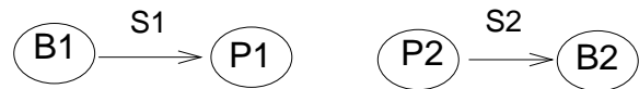
Figure 7: A two cell configuration where both pads are in range of their respective base stations and also in range of each other. Base station B1 is sending data to pad P1, and pad P2 is sending data to base station B2. Each stream is generating data at a rate of 64 packets per second and using UDP for transport.
