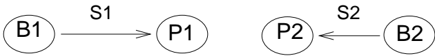
Figure 6: A two cell configuration where both pads are in range of their respective base stations and also in range of each other. The base stations are sending data to their respective pads, and each stream is generating data at a rate of 64 packets per second and using UDP for transport.
