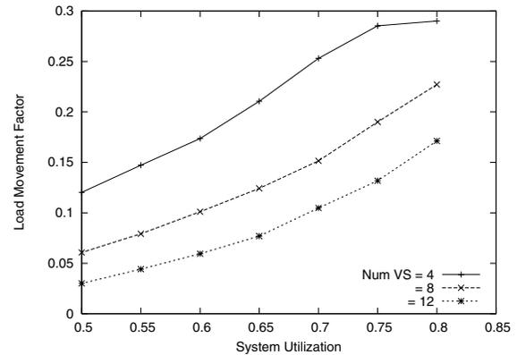
Fig. 11. Load movement factor vs. system utilization after an impulse in 10% of the ID space.
