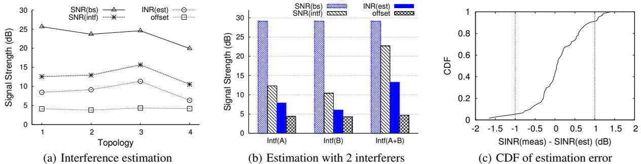
Figure 6: Accurate estimation of SINR from individual SNR estimates.
