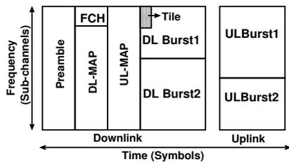
Figure 1: WiMAX frame structure.
