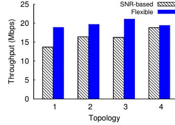
Figure 5: Joint association increases throughput by 40% comparing to decoupled (SNR based) association.
