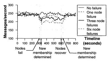
Figure 11. Reconfiguration timeline with replication.
