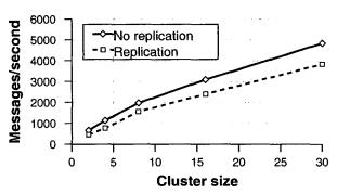
Figure 5. Throughput of the system configured with infinitely fast disks.
