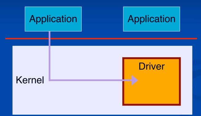
Restarting failed drivers prevents system crashes by reinitializing driver & kernel data structures
