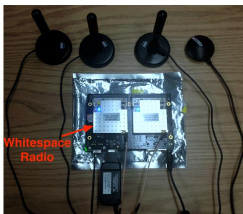
Figure 3.9: TV whitespace radios in an OpenWrt based router.
