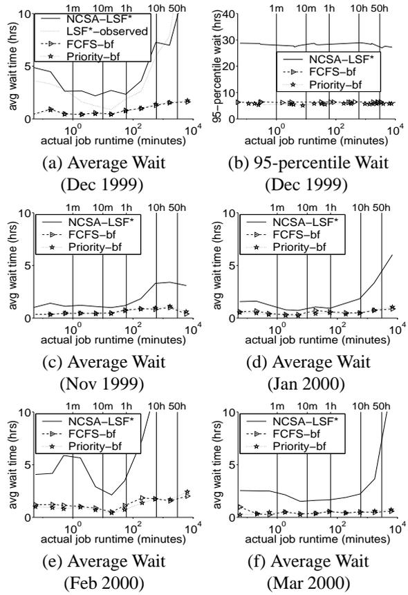
Figure 5. Performance of Priority-backfill, FCFS-backfill and NCSA-LSF\*
