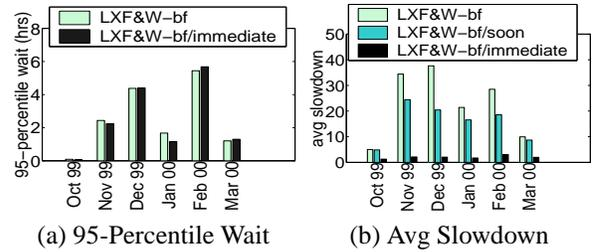
Figure 8. Performance of LXF&W-backfill with 1 Minute of Immediate Service
