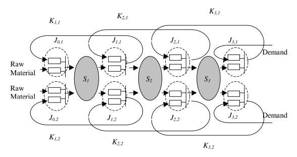
Figure 2. Queueing model representation of multiproduct kanban systems
