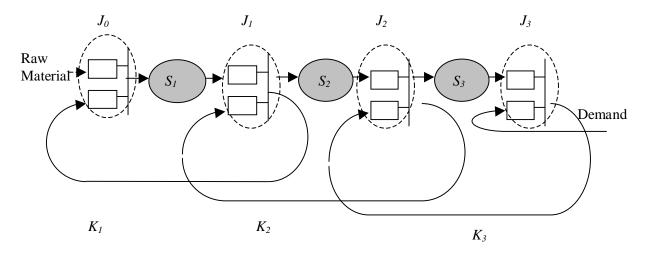
Figure 1. Queueing model representation of single product kanban systems
