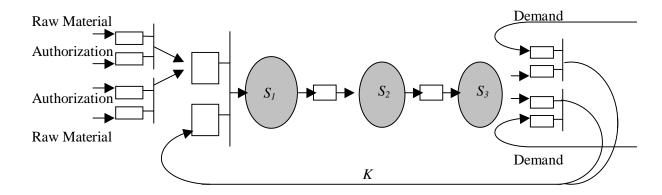
Figure 3. Queueing model representation of multiproduct CONWIP systems
