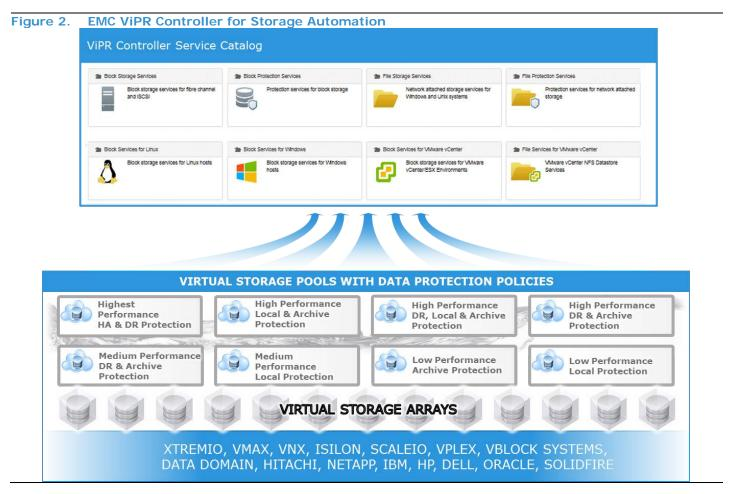
Principally, a storage device features a control path and data path. In simplistic terms, the control path sets and manages the policies for the storage device and the data path performs the actual reads, writes and services. ViPR Controller is unlike previous
