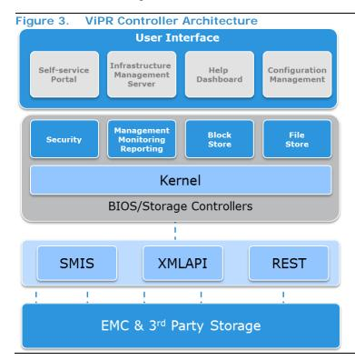
ViPR Controller guides an administrator through the process of discovering the g the storage infrastructure. Once a storage administrator adds arrays, they are automatically discovered, including all their corresponding storage pools and ports. Once the Fibre Channel switches are added, they are automatically discovered and mapped to the Fibre Channel networks. This discovery, virtualization and mapping is for EMC and non-EMC arrays as well as EMC and third party data protection including:
