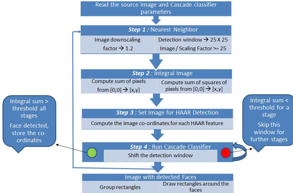
**Figure 4: Face detection implementation flow**
