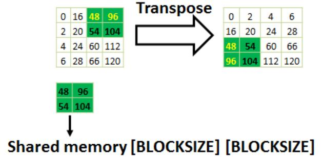
Figure 16: Naive Implementation of Matrix Transpose
