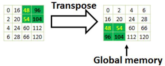
Figure 17: Optimized Implementation of Matrix Transpose
