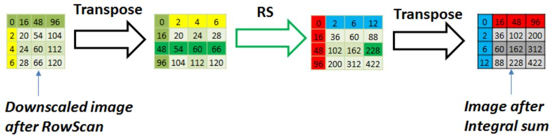
Figure 13: ColumnScan kernel breakdown
