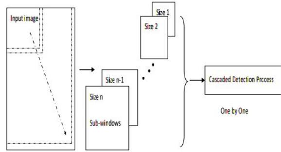
Figure 7: Scan Window Processing
