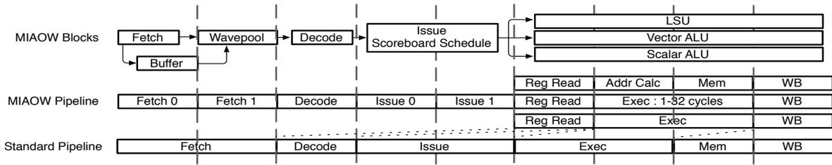
Figure 2: MIAOW Compute Unit Pipeline stages
