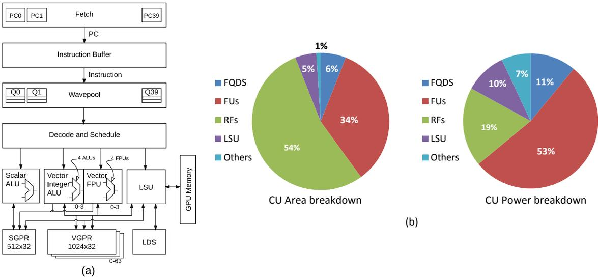
Figure 1: a) Compute Unit (CU) microarchitecture; b) Compute Unit (CU) Area and Power breakdown [FQDS: Fetch/Queue/Decode/Schedule; FUs: Functional Units; RFs: Register Files; LSU: Load Store Unit] (Area metric –  $\mu\text{m}^2$  and Power metric – mW)
