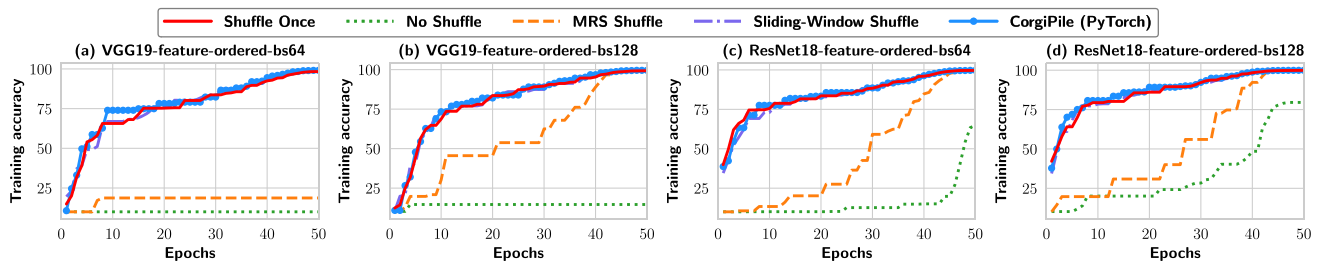
Fig. 18 The convergence rates of deep learning models with different data shuffling strategies and batch sizes, for the feature-ordered 10-class cifar-10 image dataset
