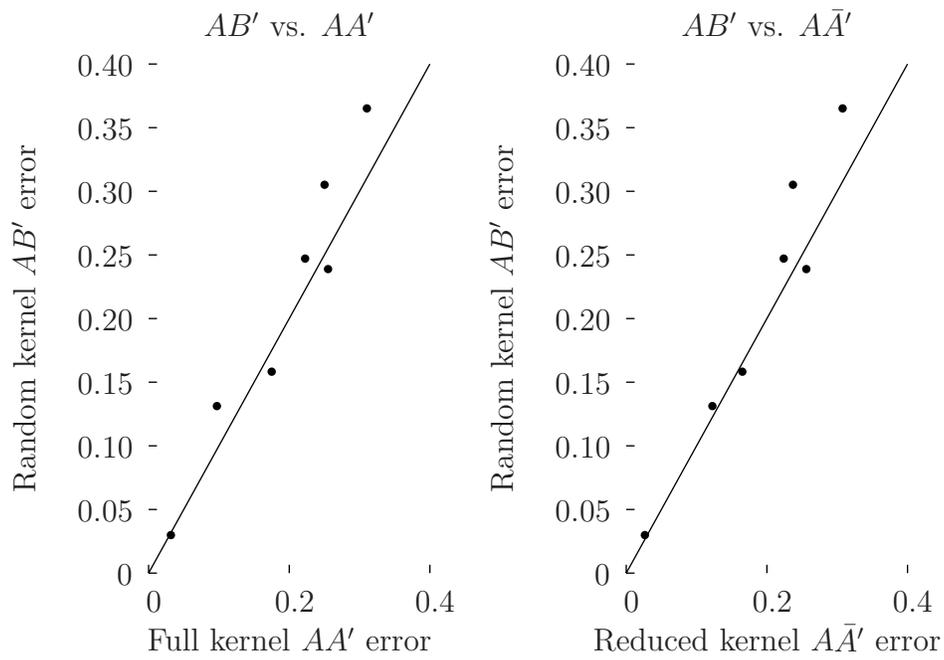
Figure 4.1 Error rate comparison of 1-norm linear SVMs for random kernel versus full and reduced kernels. For points below the diagonal, the random kernel has a lower error rate. The diagonal line in each plot marks equal error rates. One result is given for each dataset in Table 4.1.
