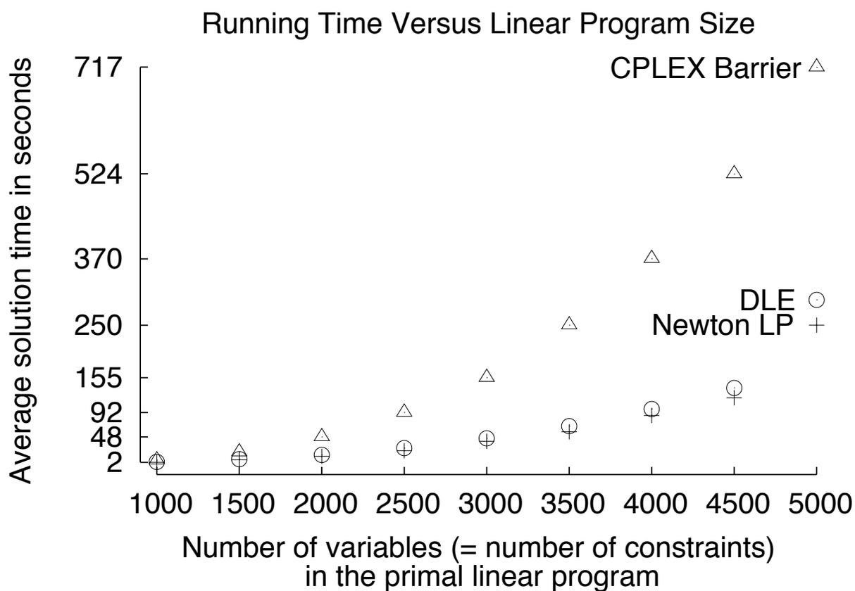
Figure 9.1 Average running times of our proposed approaches and the CPLEX 9.0 barrier method. Our Newton LP Algorithm 9.2.1 method is represented by '+', our DLE Algorithm 9.2.3 method is represented by '○', and CPLEX is represented by '△'. Each point is the average of 10 randomly generated square linear programs.
