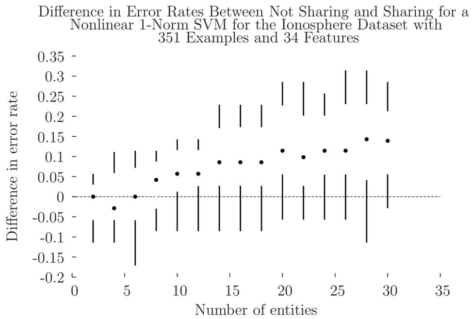
Figure 4.6 Box-and-whisker (median and interquartile) plot showing the improvement in error rate of *Gaussian* kernel PPSVM as the number of entities increases from 2 to 30.
