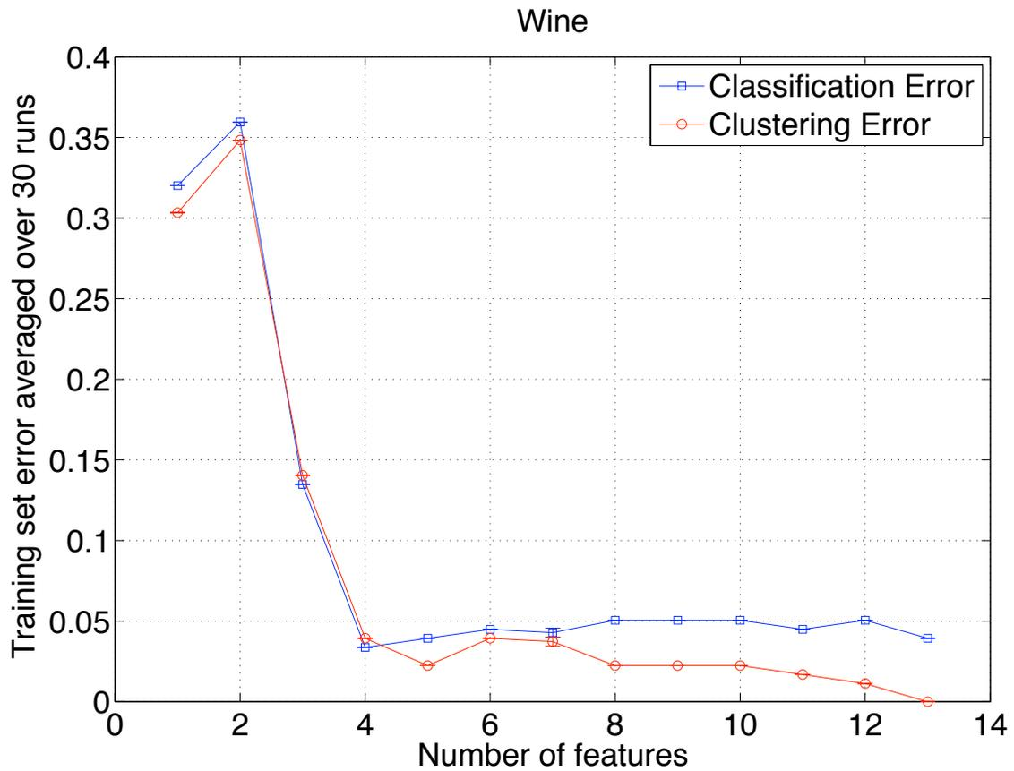
Figure 5.1 Error curves for the 3-class Wine dataset with 178 points in 13-dimensional space are plotted as a function of the number features selected by FSKM. The average range of  $\nu$  computed by (5.10) was from 42 to 55. Note that the low variance between runs on this dataset makes the error bars essentially invisible.
