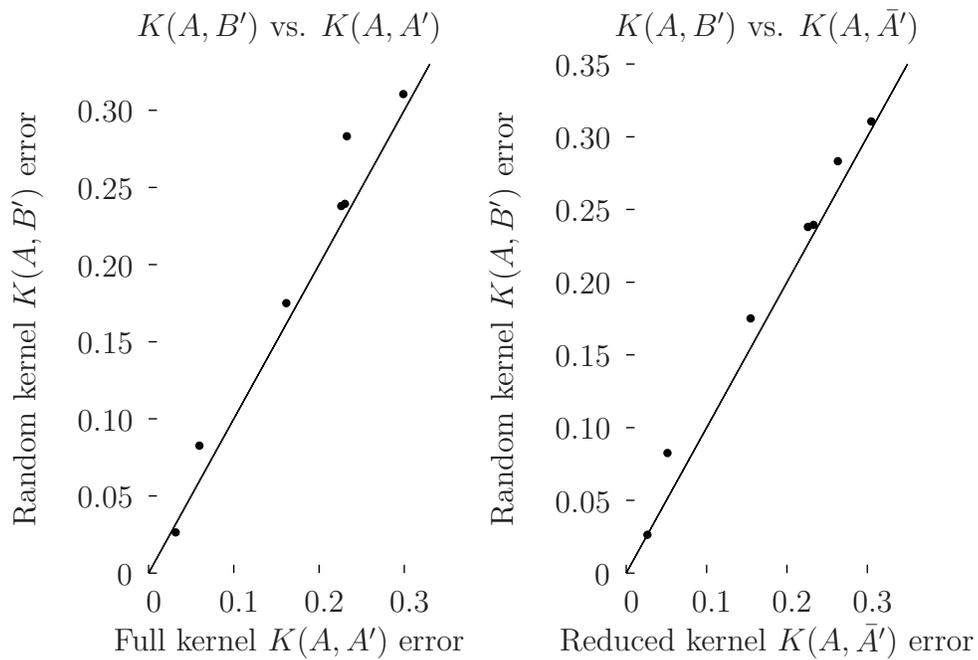
Figure 4.2 Error rate comparison of 1-norm nonlinear SVM for random kernel versus full and reduced kernels. For points below the diagonal, the random kernel has a lower error rate. The diagonal line in each plot marks equal error rates. One result is given for each dataset in Table 4.2.
