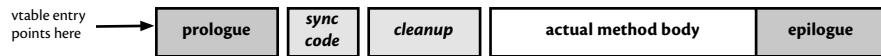
Figure 2.7: Proxy for an accessor method, with vtable pointer, synchronization point, cleanup code, and original method body.
