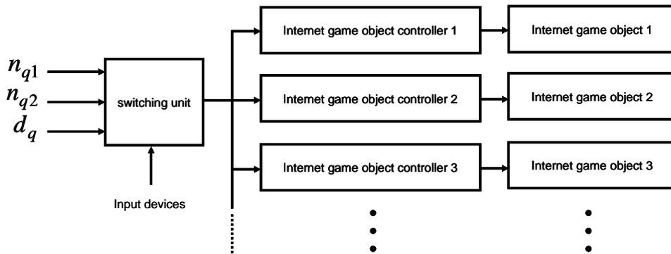
**Fig. 4.** Block diagram of the internet game object control unit.
