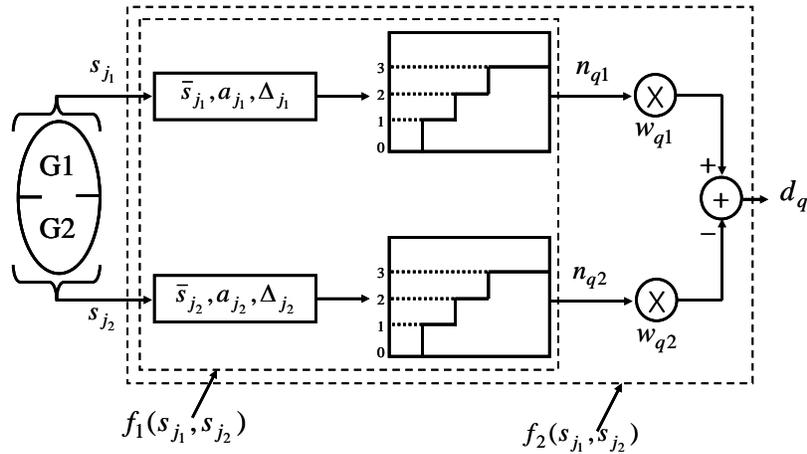
Fig. 2. Schematic diagram of the coding functions  $f_1(s_{j_1}, s_{j_2})$  and  $f_2(s_{j_1}, s_{j_2})$ .
