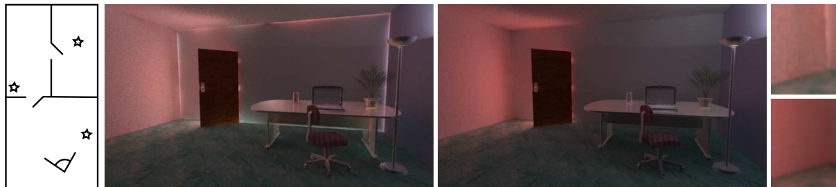
Figure 1: Leftmost is the plan of a scene in which only a small portion of the lights’ total power contributes to the image. The left image was produced using standard Photon Mapping, which under-samples some regions and over-samples others, resulting in image noise and severe energy bleeding from the adjacent room (the cause of the incorrect illumination around the edges of the rear wall). To the right is our result. Paths joining the eye to a light were sampled and photons were stored only in important locations. The insets on the far right show zoomed sections taken from the center-left of the images, and demonstrate how our method (lower) both reduces noise and avoids energy bleeding.
