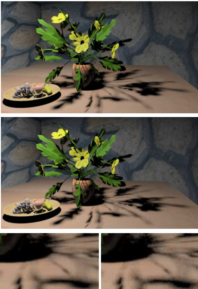
Figure 8: An image involving complex soft shadows and glossy surfaces. The top is PMC-HI sampling, while the middle is MIS with equal total sample count. Note the significant improvement in the soft shadows achieved with PMC-HI, shown in the zoomed images at the bottom (PMC-HI left, MIS right).
