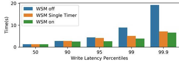
**Figure 4: Write latency percentiles for 100MB writes to S3 from AWS Lambda. Comparing WSM off, with a single timeout, and fully on**
