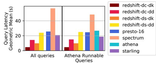
**Figure 6: Geometric mean of latency on 1TB dataset**
