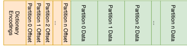
Figure 2: Starling Partitioned S3 Object Format. Metadata in orange, partitioned data in green
