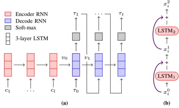
Fig. 9: **(a)** Diagram of encoder-decoder architecture for pass2path learning. **(b)** A 2-layer LSTM cells with residual connection. Here  $c_i$ 's are characters of input passwords,  $\tau_i$ 's are transitions, and  $x_i^j$ 's are internal states in neural networks.
