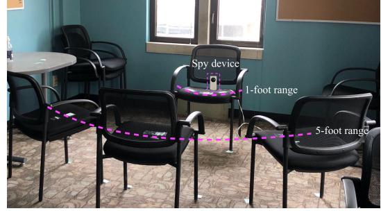
Figure 4: Our experimental setup. We created nine total equal-height place markers at 1 foot, 5 feet, and 10 feet away from a spy device and recorded each detector’s reading at each place marker. The 10 foot place markers are not shown.
