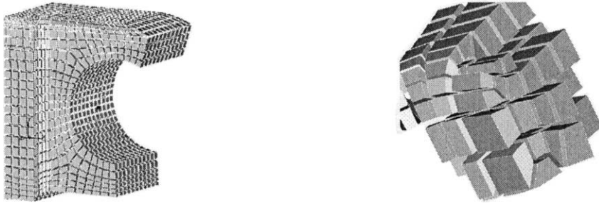
Fig. 15. Two different views on our hexahedral mesh for the most difficult part of the shovel. The right figure is a zoom into a typical detail.
