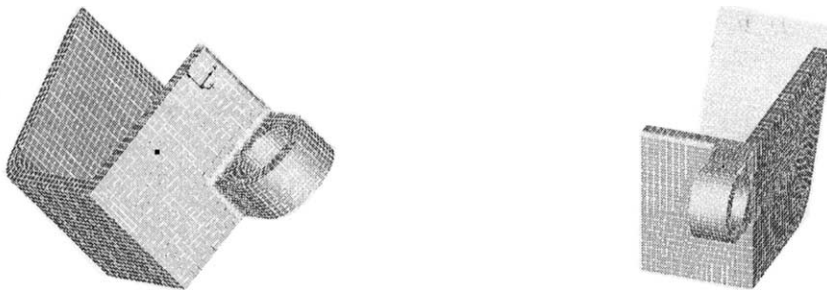
Fig. 14. Two different views on our surface mesh for a CAD model of a shovel. The surface mesh is free of self-intersecting cycles.
