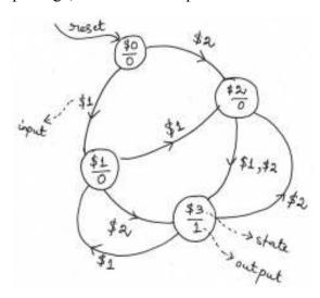
II. How many flip-flops (storage elements) will be needed to implement this finite state machine designed in your answer to part I?
