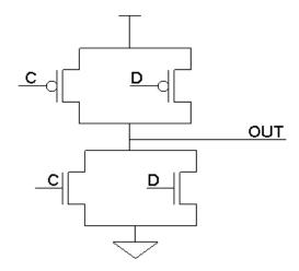
There is short circuit (path from Power to Ground) when either C = 1 and D = 0 or C = 0 and D = 1.
