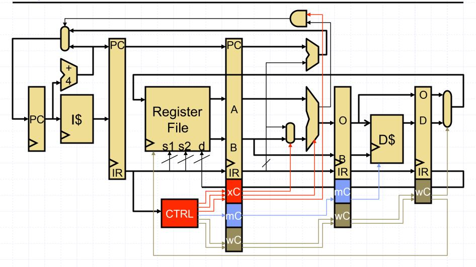
• One single-cycle controller, but pipeline the control signals
