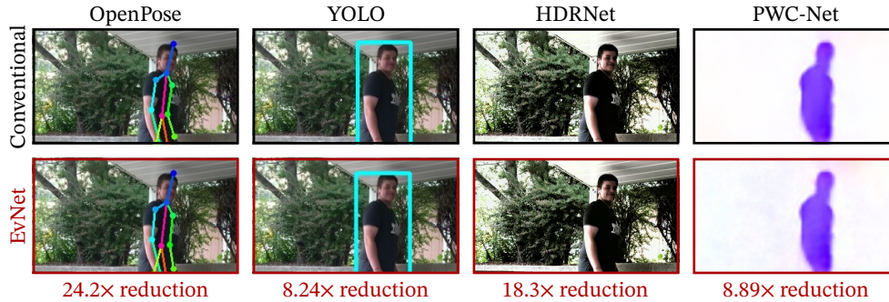
Figure 3.7: Versatility of EvNets. We demonstrate that EvNets are an effective strategy for many high- and low-level vision tasks. Across tasks, we see significant computation savings while maintaining high-quality output. This frame shows a person mid-jump. The EvNet tracks the subject correctly under rapid motion.
